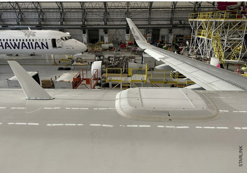
◀ A Starlink terminal after installation on a Hawaiian Airlines jets.
